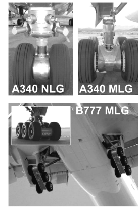
Fig. 9 Examples of landing gear add-on noise reduction fairings.
